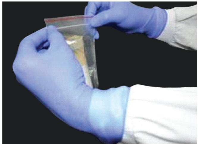
Fig. A4.4: Place the primary tube with the sample inside the Ziplock pouch covered with adsorbent material, e.g., cotton, and can be secured with a rubber band
