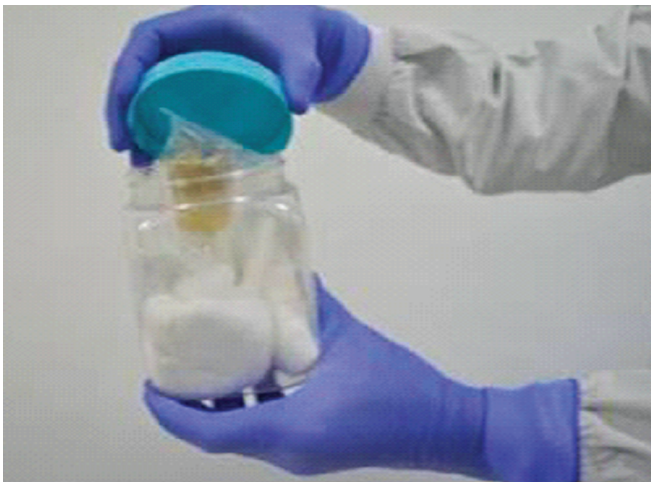
Fig. A4.5: The Ziploc pouch is kept in another plastic secondary container which is further secured
