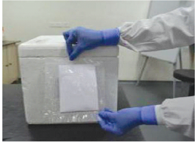
Fig. A4.8: Attaching the labels: Senders' address, contact number; Consignee's address/contact number. Biological substance - Category B; "UN 3373"; orientation label, handle with care, with a rubber band
