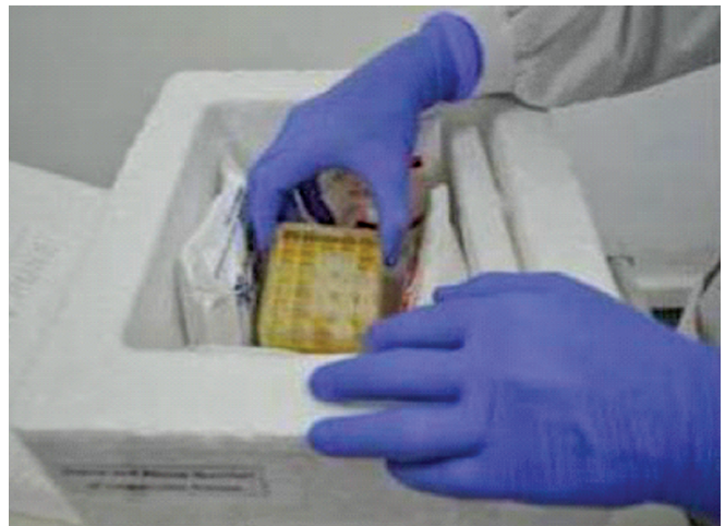
Fig. A4.6: The thermocol box is used as the outermost container and the secondary container is placed within it with frozen gel packs surrounding it
