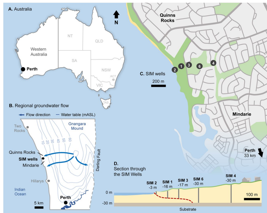
Figure 3. Maps providing location and characterisation of the Quinns Rocks seawater intrusion monitoring (SIM) reference site in Perth, Western Australia. (A) The location of Perth relative to Western Australia. (B) The regional groundwater contours, which are approximately parallel to the coastline at Quinns Rocks indicating groundwater flows towards the coast. (C) The location of the SIM wells relative to Quinns Rocks, which have been monitored since 1990. (D) A cross-section of the SIM wells, including the impermeable clayey substrate and an estimate of the current position of the seawater wedge.
