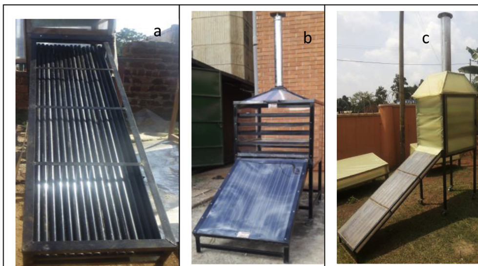
Figure 2. The new proposed improved solar dryer (ISD) for tropical fruits. a) the multiple metallic solar thermal energy concentrators, b) the ISD with a modified solar concentrator, c) full ISD with cabinet enclosed with greenhouse cover.
