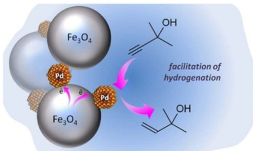
Figure 9. Fabrication of magnetically recoverable catalysts based on mixtures of Pd and magnetite nanoparticles for hydrogenation of alkyne alcohols. Reprinted from Ref. [173]. Copyright 2014 American Chemical Society.
