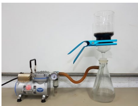
Figure 2. Experimental setup of vacuum filtration.
