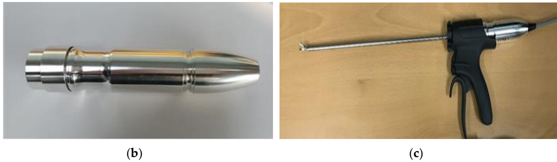
Figure 6. (a) 3D model and (b) assembled outer case part. (c) Assembled BLUT, waveguide, and handheld instrument.
