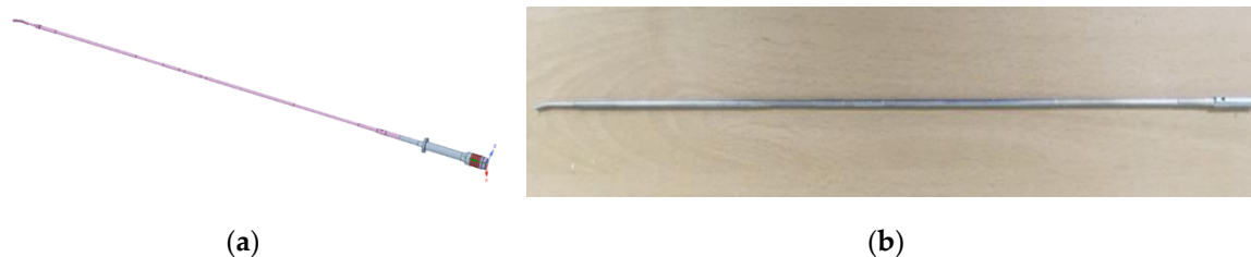
Figure 3. (a) A model 36 cm waveguide in the handheld instrument; (b) a fabricated 36 cm waveguide.
