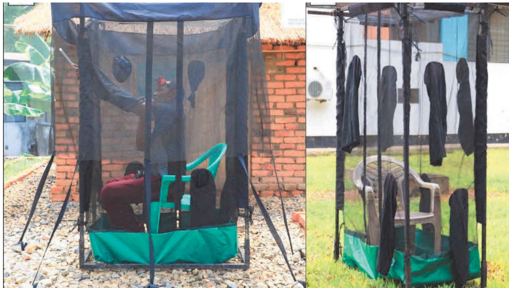
Fig. 2 Photo of the miniaturized double net trap used to catch host-seeking mosquitoes indoors and outdoors. The miniaturized double net trap consists of an inner chamber, normally occupied by adult volunteer mosquito catchers. There is an outer netting cover, hanging 80 cm from the ground, which traps host-seeking mosquitoes attempting to reach the volunteer inside. Host-seeking mosquitoes are trapped between the inner and outer netting compartments are collected by the volunteer through the multiple sleeves which open outwards from the inner compartment using a mouth aspirator
