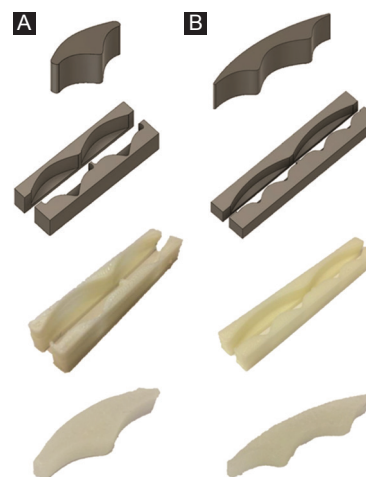
Figure 3. The computer-aided design of patch molds for (A) 2-tooth model and (B) 3-tooth model for three-dimensional printing and their respective final products.
