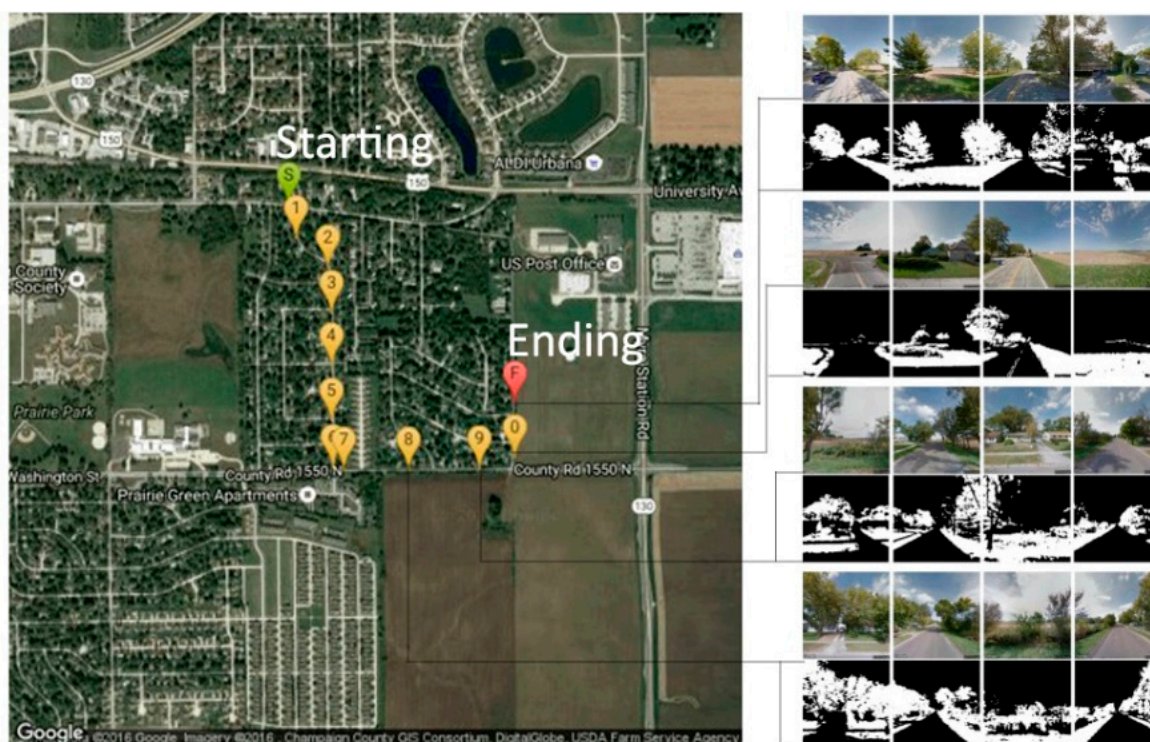
Figure 1. Green Index on A Route: S is the starting point and F is the ending point of the route. We extracted 4 street view images every 20 m along the route. For each image, the percentage of green pixels is calculated which is the vegetation density.
