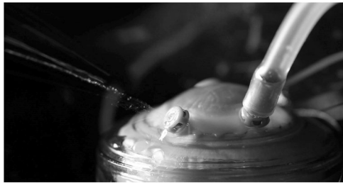
Fig. 5 Droplets from failed valved cannula. Photograph of droplets vented from a failed valved cannula at the beginning of fluid-air exchange to videos.
