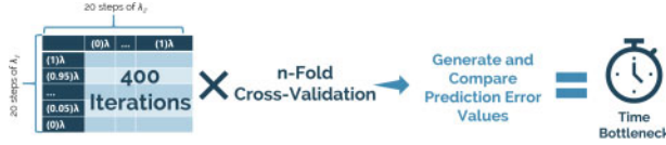
Fig. 2. The time bottleneck due to the serial nature of the original EBEN algorithm
