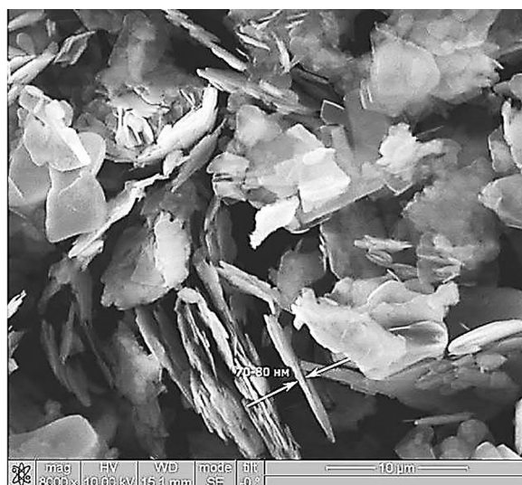
Figure 10. SEM of h-BN particles after APTES treatment.
