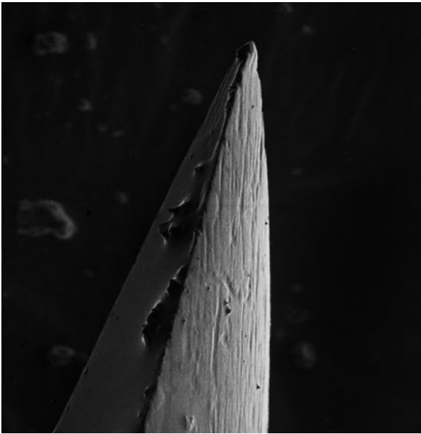
Fig. 2 Control sample showing undamaged bevel tip (500x).
