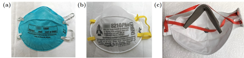
Fig 4. Masks after 5 heat cycles. A: 3M 1860; Slight blurring of printed label, no other visible changes. B: 3M 8210 Plus; Slight blurring of the printed label. C: 3M 1870; Delamination of part of the foam nose bridge shown here after 5 cycles. The foam was reset in place prior to donning and still passed all fit tests.
