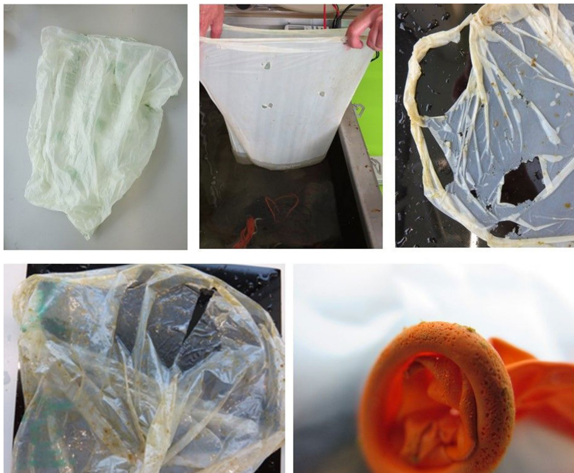
Figure 3. Pictures of fragmentation of compostable trash bag 7P0069 after 0, 57 and 183 days from left to right, respectively (upper panels), compostable postal bag 7P0059 after 294 days (lower left panel) and latex balloon after 383 days (lower right panel) in the microcosm.
