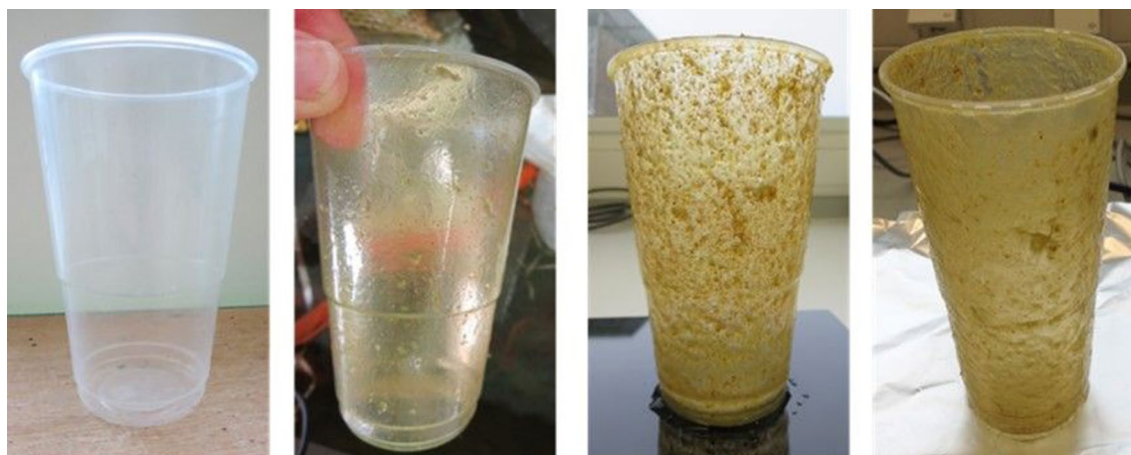
Figure 6. Biofouling of polypropylene cup, after (from left to right) 0, 57, 183 and 390 days in the microcosm, respectively.
