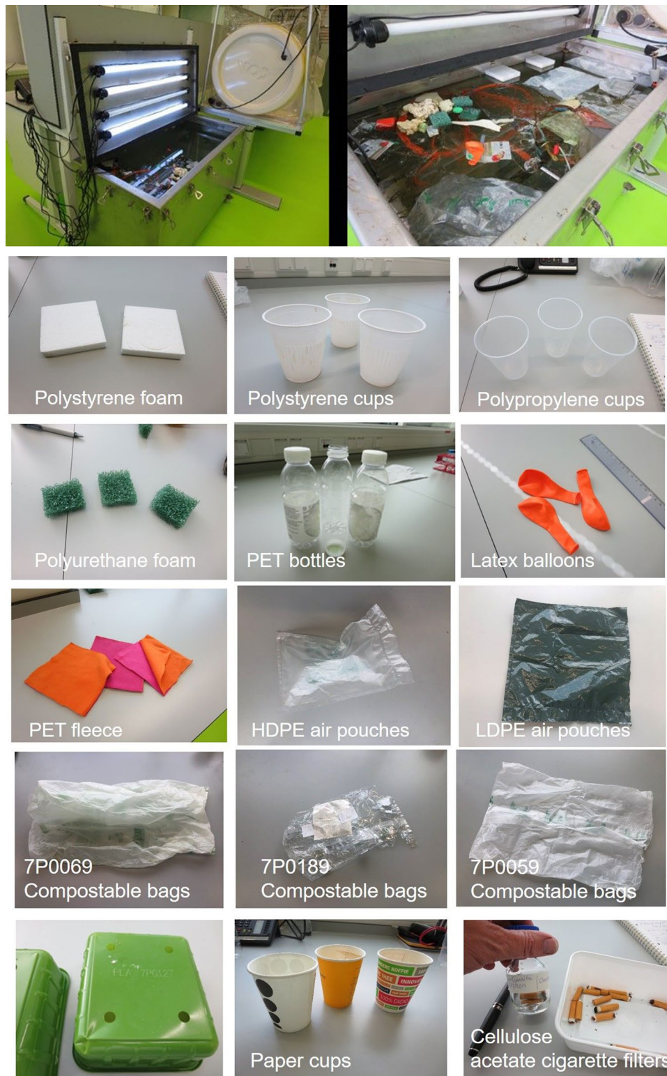
Figure 1. Pictures of (A) the marine microcosm and (B) added plastic objects with different polymer backbones.
