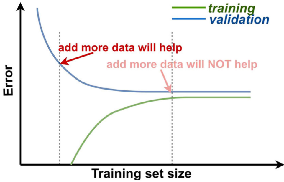
Fig. 3. The learning curve example for diagnostic purpose of data size.
