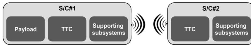
Fig. 52. Example of a space-based network. The two light gray boxes represent two spacecrafts, connected through a high-capacity communication system. Each one of them is composed of different modules, e.g. the Telemetry, Tracking and Command (TTC): when one of them fails, the corresponding spacecraft can rely on the other to backup that function, and to fulfill its mission.
