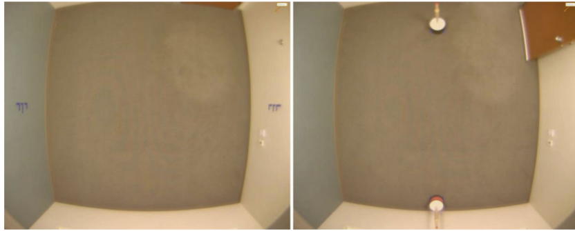
Fig. 7. Example of calibration points on the wall (left) and calibration points created using two columnar structures (right).
