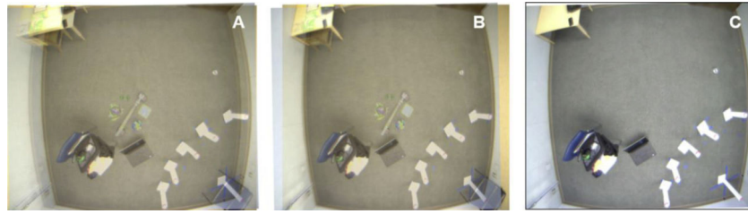
Fig. 11. Steps to fixing a frame shift, including rotation (A), translation (B) and final cropped image (C).
