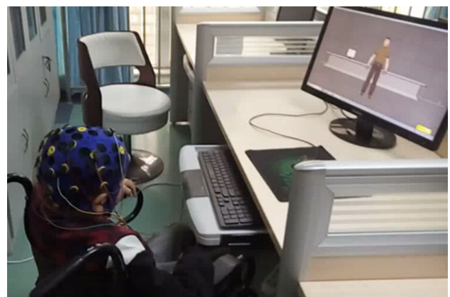
Fig. 3 An EEG based virtual rehabilitation training system. In this virtual rehabilitation system, the subject uses motor imagery paradigm to control the hand movement of the virtual man on the screen by EEG signals. The system is used to assist in the rehabilitation training of hand movement disorders, and can provide the real-time visual feedback to the subject
