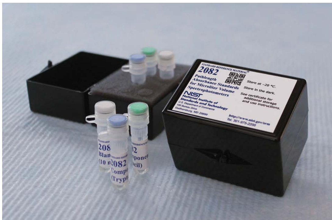
Fig. 1. Packaging of SRM 2082 showing the TRIS buffer, component A (tryptophan), and component B (uracil).
