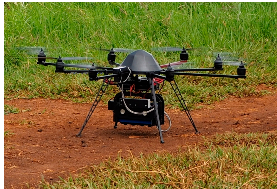
Figure 3. Mikrokopter OktoXL 6S12 unmanned aerial platform equipped with the micro-MCA12 Tetracam multispectral sensor, showing the placement of the Incident Light Sensor (ILS) module with white diffusor plate connected by a fiber optic cable to the top of the UAV facing upwards while the other 11 multispectral sensors are positioned on a dual axis gimbal camera platform for zenithal/nadir image capture. The RGB (Red-Green-Blue) and TIR (thermal infrared) cameras were alternately mounted on the same gimbaled platform for image capture.
