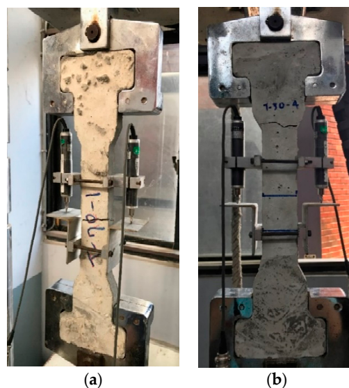
Figure 14. Failure mode of direct tension test. (a) Typical failure and (b) unexpected failure.
