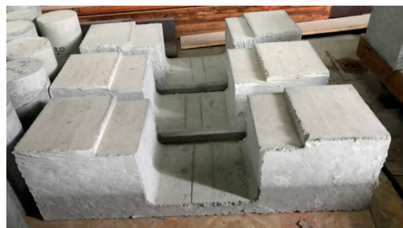
Figure 8. Cured strut-and-tie beam specimen.
