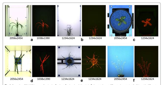
Fig. 1 Examples of FLU/VIS images of maize (a, d), wheat (b, e) and arabidopsis (c, f) shoots taken at different phenotyping facilities with different camera views (side/top) and spatial resolutions
