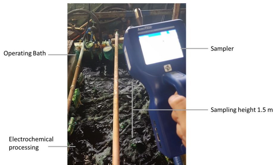
Figure 1. Sampling of industrial aerosol particles in the electroplating workshop. H = 1.5 m (Example).
