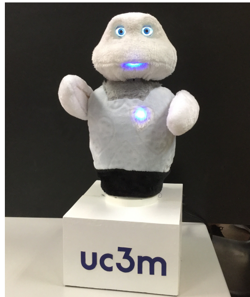
Figure 1. Mini, a social robot developed for interacting with older adults that suffer from mild cases of cognitive impairment.
