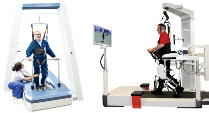
Figure 3. Robot-assisted gait trainer. Lyra (Thera Trainer, Hochdorf, Germany) (left); Lokomat (Hocoma, Volketswil, Switzerland) (right).
