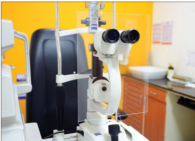
Figure 2: Breath shield for the slit lamp made using a thick transparent plastic sheet
