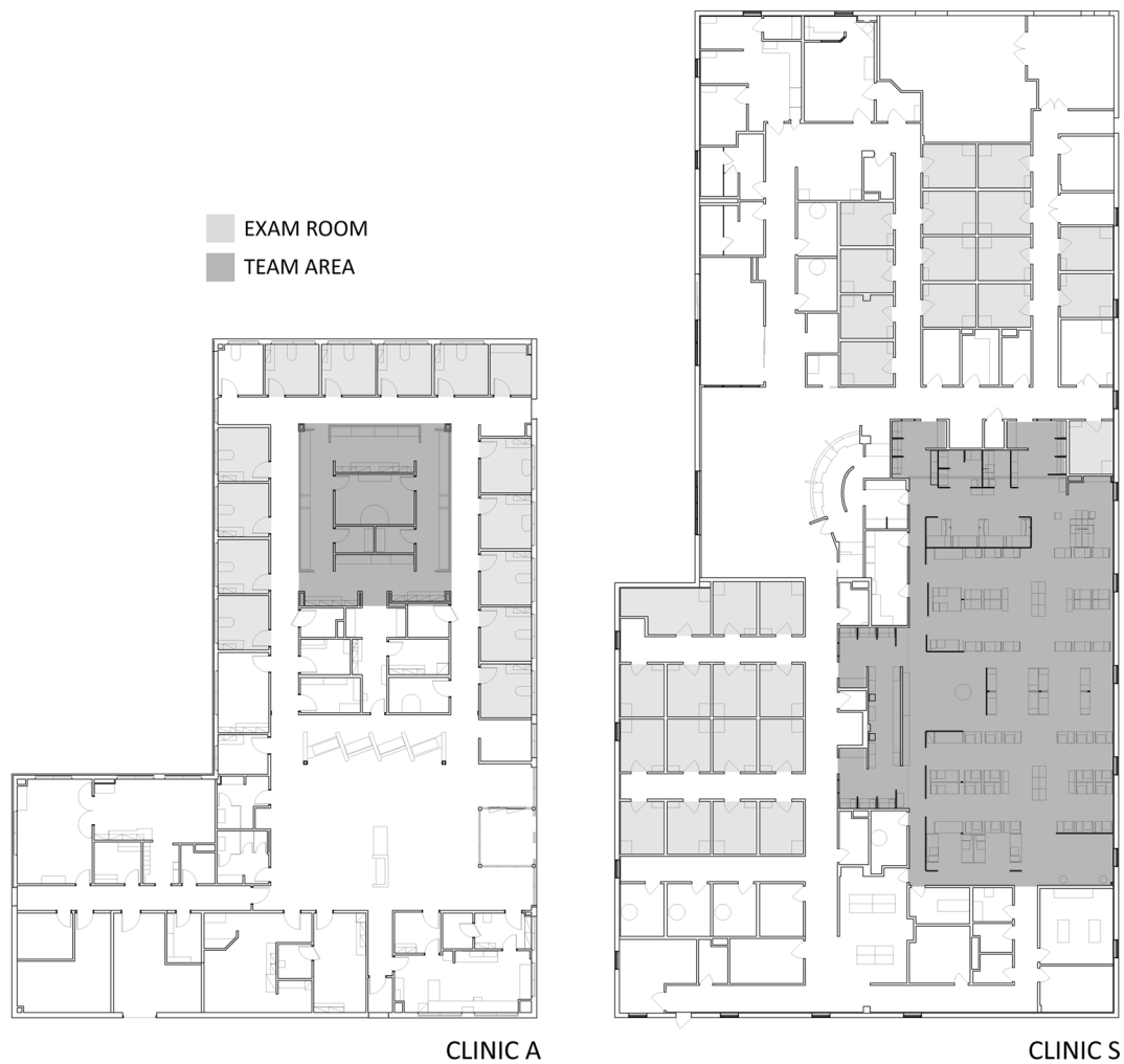
Figure 2 Layouts of the two clinics (left: Clinic A, right: Clinic S). Clinic A's team workspace is adjacent and open to patient circulation, and Clinic S's team space is a large central room separate from patient circulation and the exam rooms.
