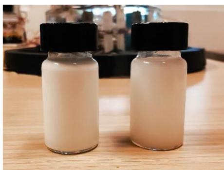
Figure 2. Suspensions of \text{TiO}_2 in DIW with volume concentration of 4% (left) and 2% (right).
