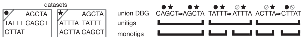
Fig. 2. Left: 2 datasets and their k -mers ( k = 5 ). Right: a union DBG is built over these k -mers, and contains 3 unitigs (top row). Symbols (e.g. circle, star) above each k -mer symbolize the per-dataset abundances. In the left-most unitig, the two k -mers have the same abundance information. Thus the monotig is here equivalent to the unitig. In the center and right-most unitigs, k -mers that have contrasted abundances share a k - 1 overlap and can be compacted. On the contrary, monotigs will stop at differences between the coverage profiles of overlapping k -mers
