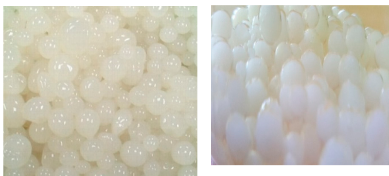
Figure 5. Gellan gum microbeads of Enterobacter sp. strain BRC05 before and after 24-h cycle degradation.
