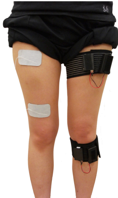
Fig. 2. Nine-axis sensors were attached to the thigh and lower leg of the non-affected side. The quadriceps femoris muscle was stimulated using functional electrical stimulation. The stimulation points were based on the motor points.
