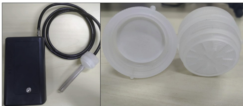
Fig. 2. MA200 carbonaceous particle monitor with the holder containing the CA/CPB nanofiber.
