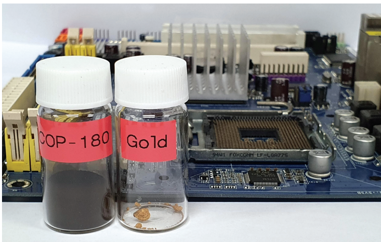
Porous porphyrin polymer (COP-180) can extract gold from a computer circuit board and produce pure gold nuggets.
