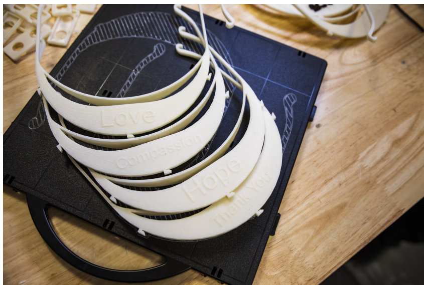
Figure 1. 3D printed face shield visor manufactured in our laboratory to support national coalition efforts. Design: Stratasys' three hole punch spacing visor. Machine: Fortus 250 mc. Material: acrylonitrile butadiene styrene.
