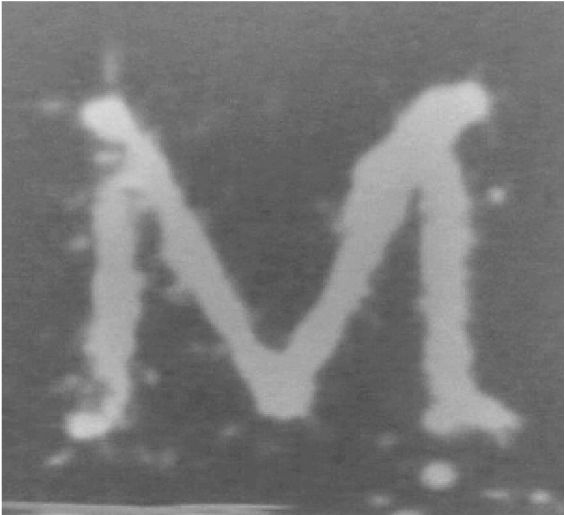
Fig. 8. An image showing a patterned lesion in the shape of a 1 cm wide block 'M' generated through Skullcap 3 by mechanically repositioning the skullcap with respect to the transducer to generate the lesion. This lesion was generated by applying histotripsy pulses through the skullcap without using aberration correction.
