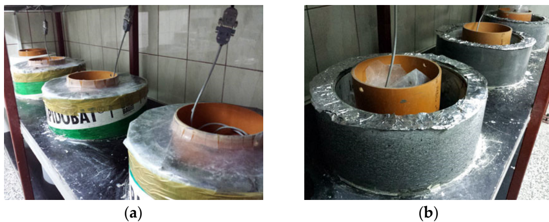
Figure 9. Restrained shrinkage test of concrete: (a) concrete samples insulated and subjected to autogenous shrinkage; (b) side formwork removal after 24 h of concreting and measurement of the impact of the drying shrinkage.
