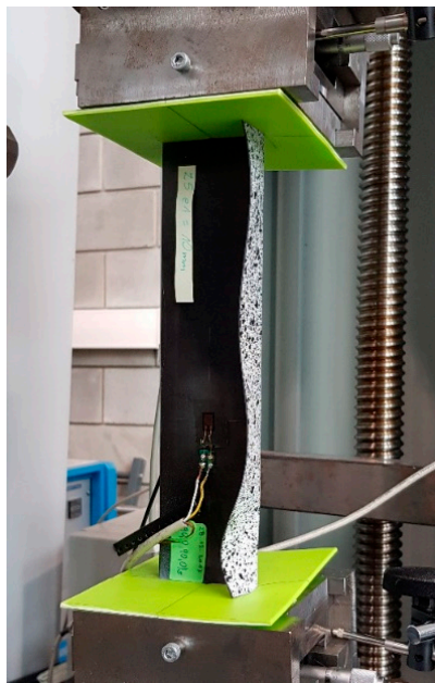
Figure 9. Buckling mode of the structure under the load eccentricity e_1 = 10 mm: (a) experimental; (b) numerical.
