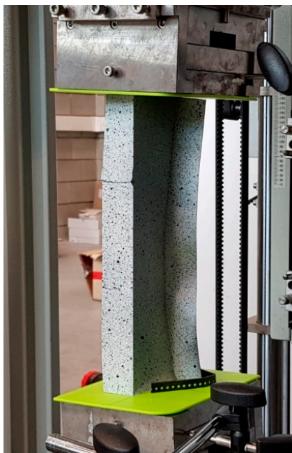
Figure 9. Buckling mode of the structure under the load eccentricity e_1 = 10 mm: (a) experimental; (b) numerical.
