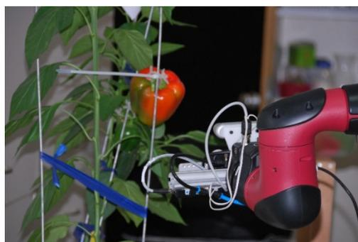
**Figure 5.** Camera mounted on the robot to acquire images of a red pepper fruit mounted on a pepper plant.
