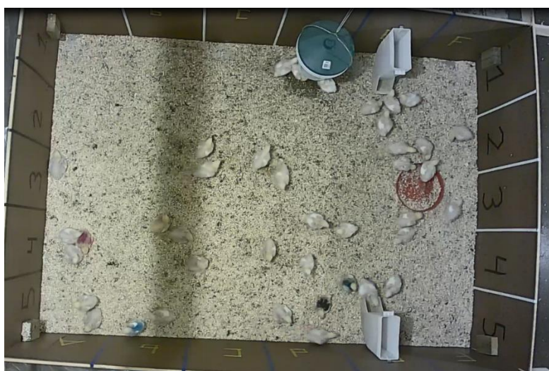
Figure 2. Top view of the tracking pen during this study, with bedding on the false floor underneath which the RFID antennas are situated. Lines on the pen walls indicate the position of the antenna grid.
