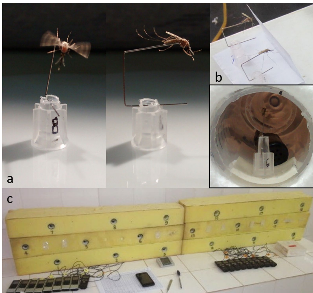
Fig. 2 Tethered female Anopheles gambiae s.l. a Entomological pin attached to ventral side of posterior abdomen of the mosquito ( a ; right), allowing unobstructed flight ( a ; left). Bottom part of pin inserted into clipped 10 µl pipette tip as a base. b Tethered mosquitoes in recuperation time before assay start, fore legs resting on folded paper for tarsal contact preventing flight. c Tether flight hive of 18 flight tubes housed inside soft (mattress) foam for surrounding sound muffling and external cue reduction. Each flight tube microphone connects to an individual sound recorder. c , Tethered female inside flight tube (polystyrene prototype, not used in the experiment); tethered mosquito construct attached on to double-sided foam tape with microphone (black) in backdrop. Photos by: RF ( a and c ) and ASY ( b and c )
