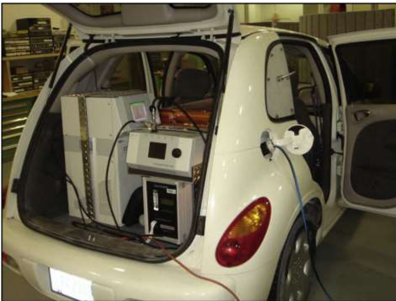
Figure 1. EPAs all-electric GMAP vehicle outfitted with various sampling instrumentation.
