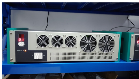
Figure 15. Battery test system CDS-SY200A-T02. "Photograph courtesy of "Renzheng Li". Copyright 2020."
