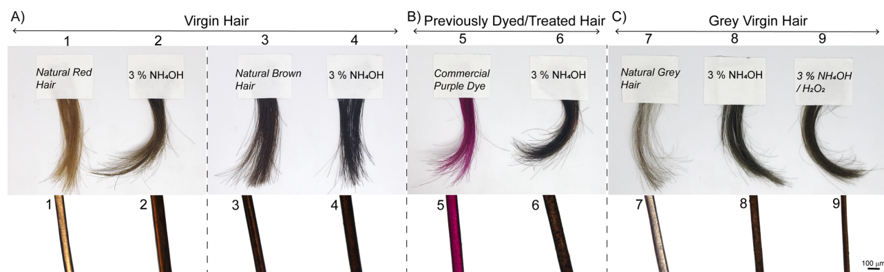
Figure 7. Polydopamine deposition is compatible with a wide range of hair substrates. (A) Natural virgin red (1) and brown (3) hair and (B) hair dyed with a purple hair dye (5) were used as hair substrates. Dopamine oxidation was carried out using 3% \text{NH}_4\text{OH} as shown in Figure 2. (C) Virgin gray hair (7) was dyed using 3% \text{NH}_4\text{OH} (8) and 3% \text{NH}_4\text{OH}/100\ \text{mM}\ \text{H}_2\text{O}_2 (as for sample 5 in Figure 4). In every case, reactions were carried out at 37\text{--}40\ ^\circ\text{C} for 2 h and hair samples were washed five times with water and three times with a 10% shampoo solution prior to imaging/analysis.
