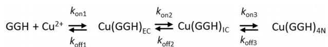
Scheme 1. The proposed mechanism of \text{Cu}^{\text{II}} reaction with GGH yielding the 4N complex and definitions of accompanying rate constants.
