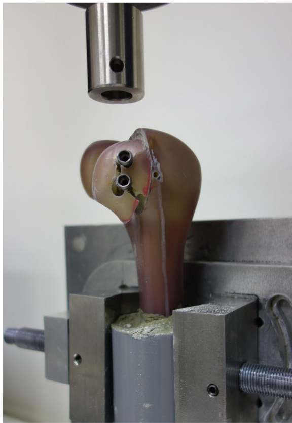
Fig. 4 The Hoffa fragment was displaced distally from its original position. Most of the constructs failed as the screw dislodging accompanied with cortex disruption
