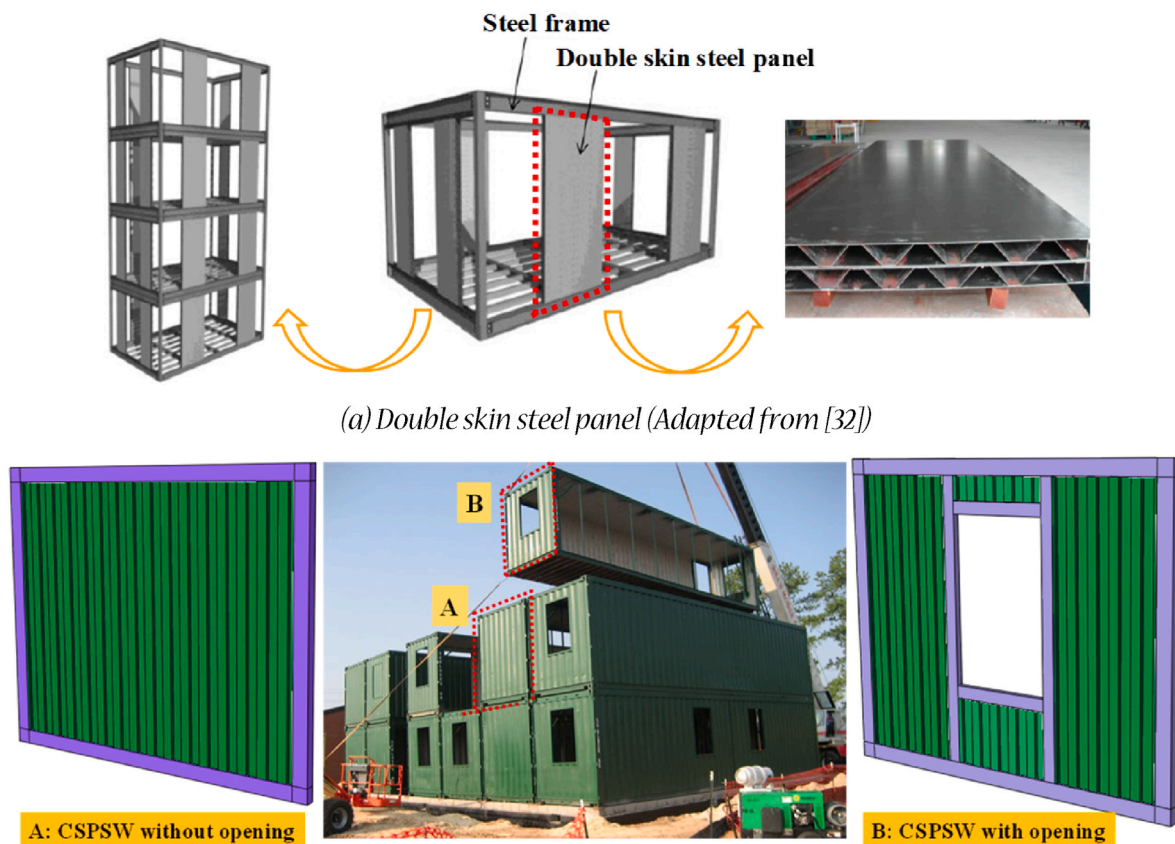
(a) Double skin steel panel (Adapted from [32])
