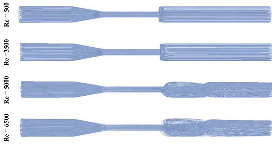
Figure 8: 1635 pathlines in FDA nozzle for different flow regimes.
