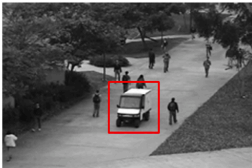
(a) Example of anomaly in the UCSD Pedestrian dataset [30]. Cars are not allowed in the pedestrian path, so the behaviour is anomalous in terms of appearance.
