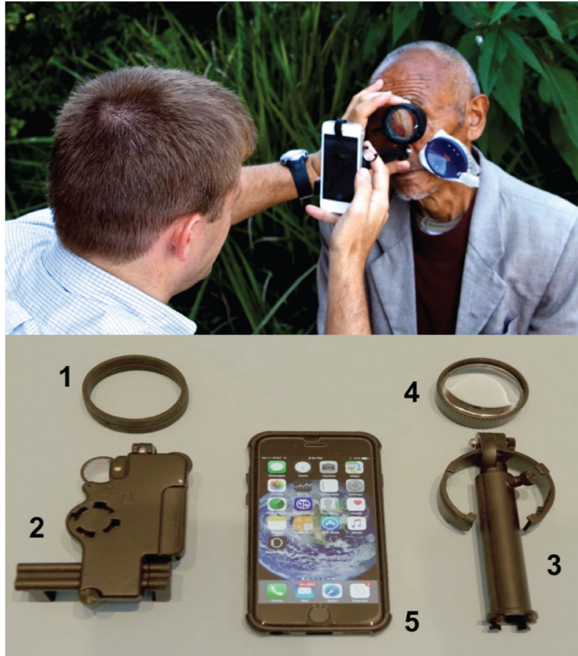
Figure 1: Upper: An ophthalmologist using the Paxos Scope mobile ophthalmic camera by Verana Health (San Francisco, CA, USA). Lower: The Paxos Scope components: 1-Flexible lens adaptor, 2-Anterior Adaptor, 3-Posterior Adaptor, 4-20D Lens, 5-iOS device by Apple, Inc. (Cupertino, CA, USA).
